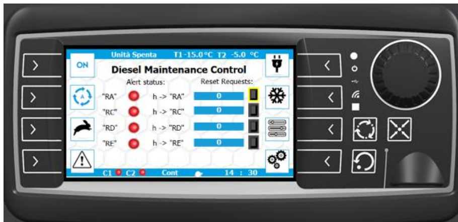
Figure 33 – Maintenance Control – road intervals
