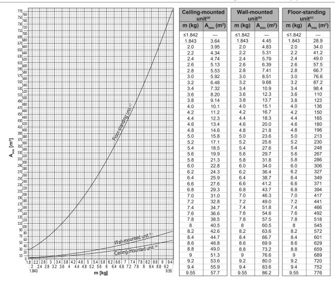
$\boldsymbol{m}\quad \text{Total refrigerant charge in the system}$
